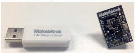
1 Plug the 2.4G Module to your robot, and turn on the power switch.
