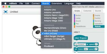
3 (Optional) From the "Connect" menu, select "Upgrade Firmware". Wait until the upgrade is complete. This will allow the mBot to talk with the computer.
