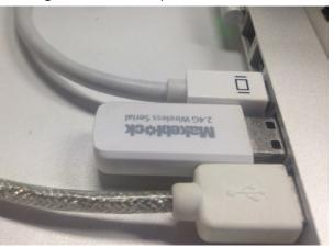
4 After that, the light on the 2.4G Module should be lighten on Steadily. Select "Connect, 2.4G Serial, the Connect" from the top menu.
