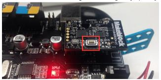
While the LED light on top of the 2.4G module is blinking quickly, plug the 2.4G Dongle into the computer.
